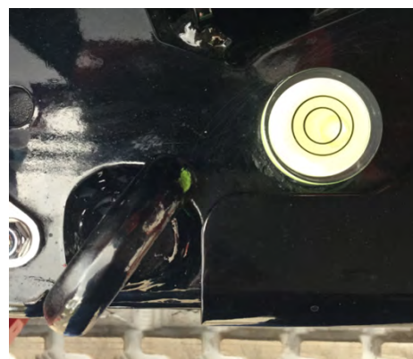
Figur 4.7 Levelling the crane
