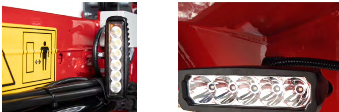
Figuur 2.12 Two work lights on the crane
